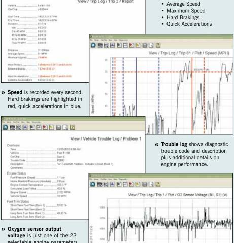
» Oxygen sensor output voltage is just one of the 23 selectable engine parameters you can choose to monitor.
